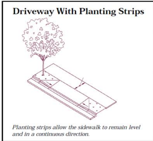
Figure 5. TMC 18.28260.C. requires driveways in the TUC to be level with the height of the sidewalk.
