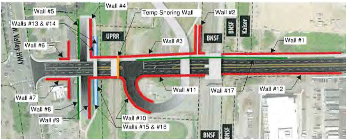
Figure 3 – Preliminary Retaining Wall Layout
