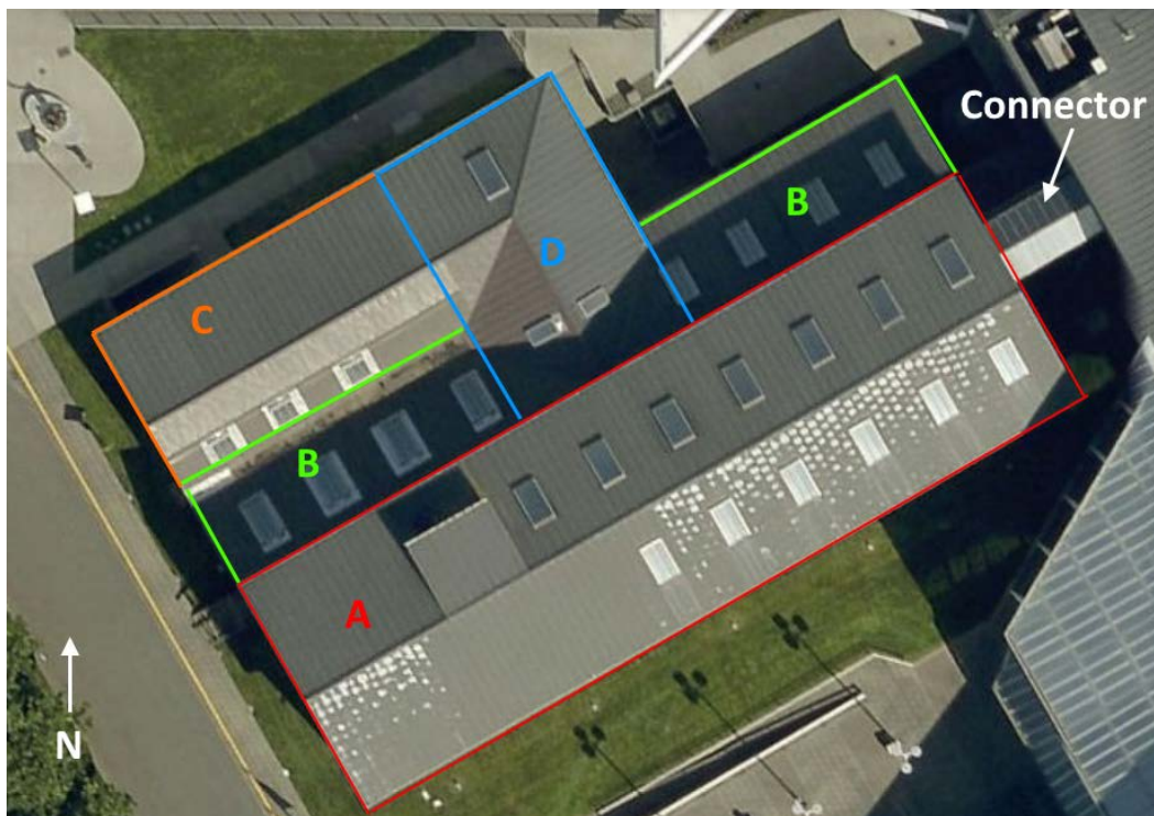
Figure A4. Red Barn. Section A is the main two-story gable structure. Section B is a one-story shed roof wing. Section C is a one-story gable wing. Section D is an intersecting, one-story gable wing. King County iMap, Aerial 2015.
