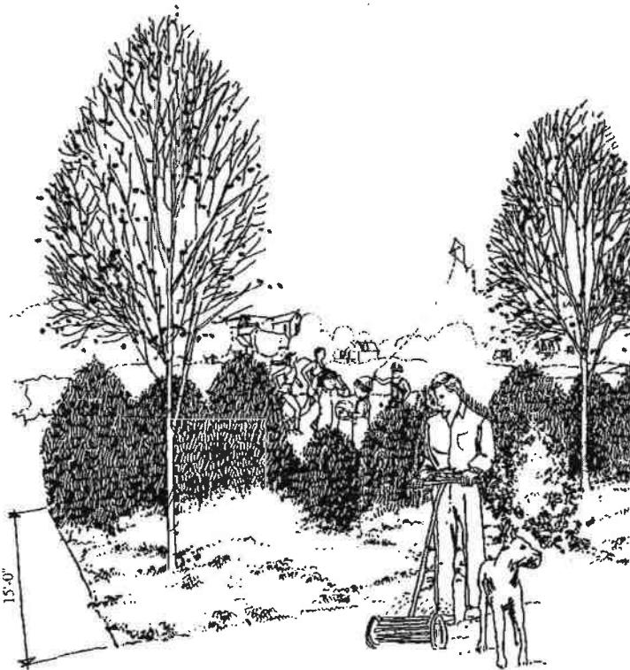
Fig. 36: Separation of marginally compatible uses with only plants.
