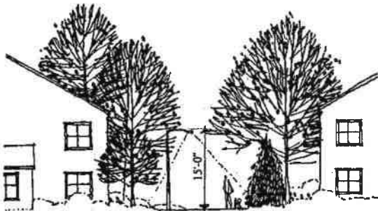
Fig. 42: Maximum grounds lighting standard height is 15 feet.
