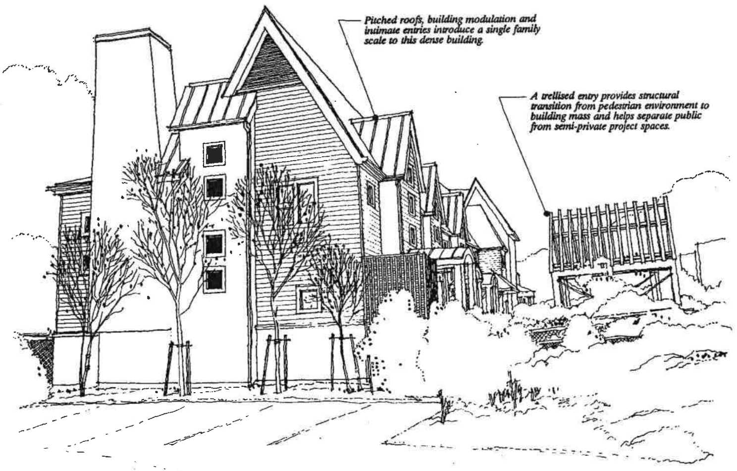
Fig. 28: Offsets, changes in materials, and other fine detailing are used to provide architectural interest.
