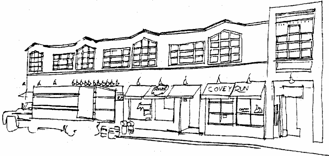
Figure 39: The roofline, windows, and details of this building break up the facade of an otherwise horizontal building. Note how the awnings and lights provide human scale while their repetition relates back to the building massing.
