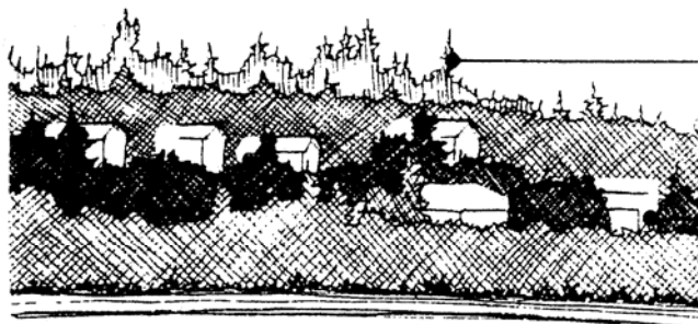
Figure 15: Horizontal building modulation. Following topography helps building mass conform to terrain.
