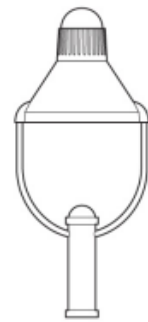
Pedestrian Post-top Luminaire
