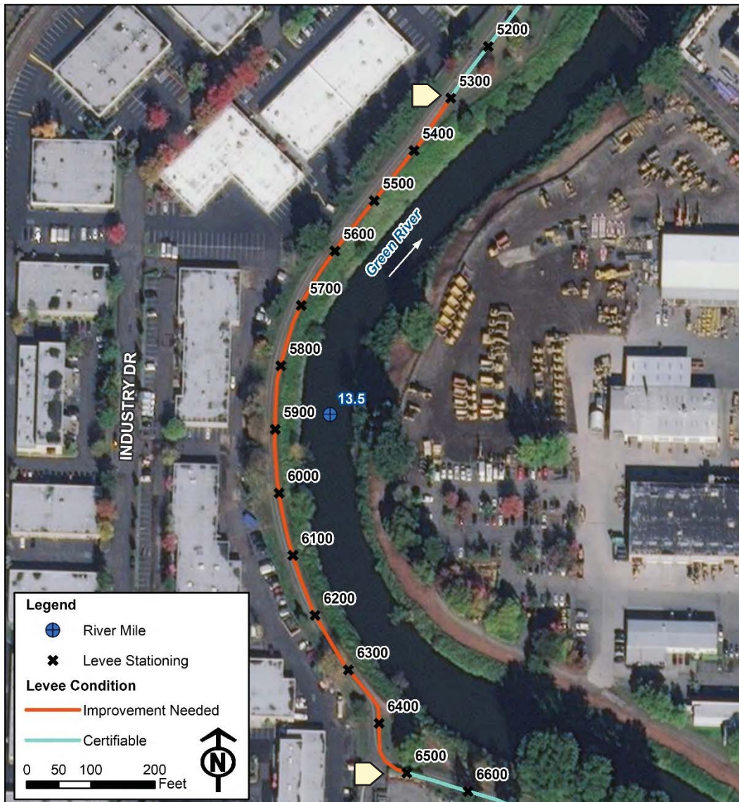
Figure 12. Tukwila Levee segment 5300 through 6500 that can't be certified in its existing condition.
