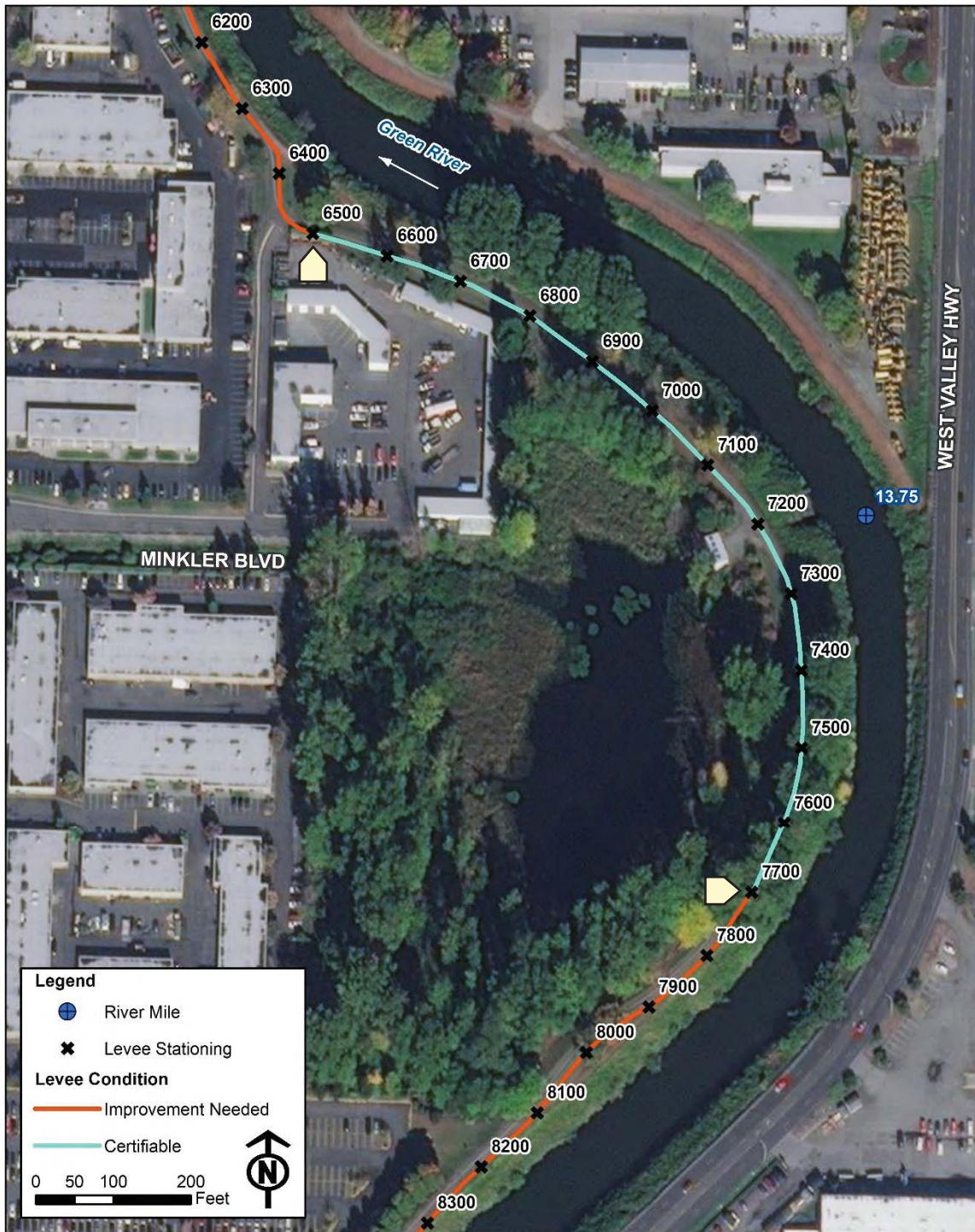
Figure 8. Tukwila Levee segment where existing section 6500 to 7700 can be certified.
