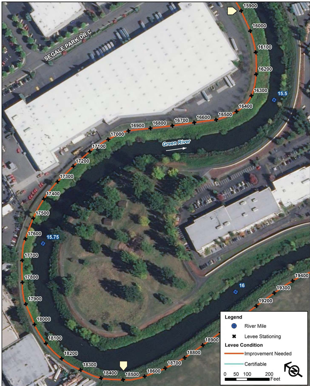
Figure 17. Tukwila Levee segment 15900 through 18500 that can't be certified in its existing condition.
