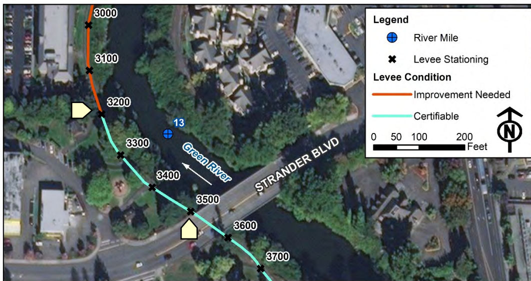
Figure 6. Tukwila Levee segment where stationing 3200 through 3500 can be certified.
