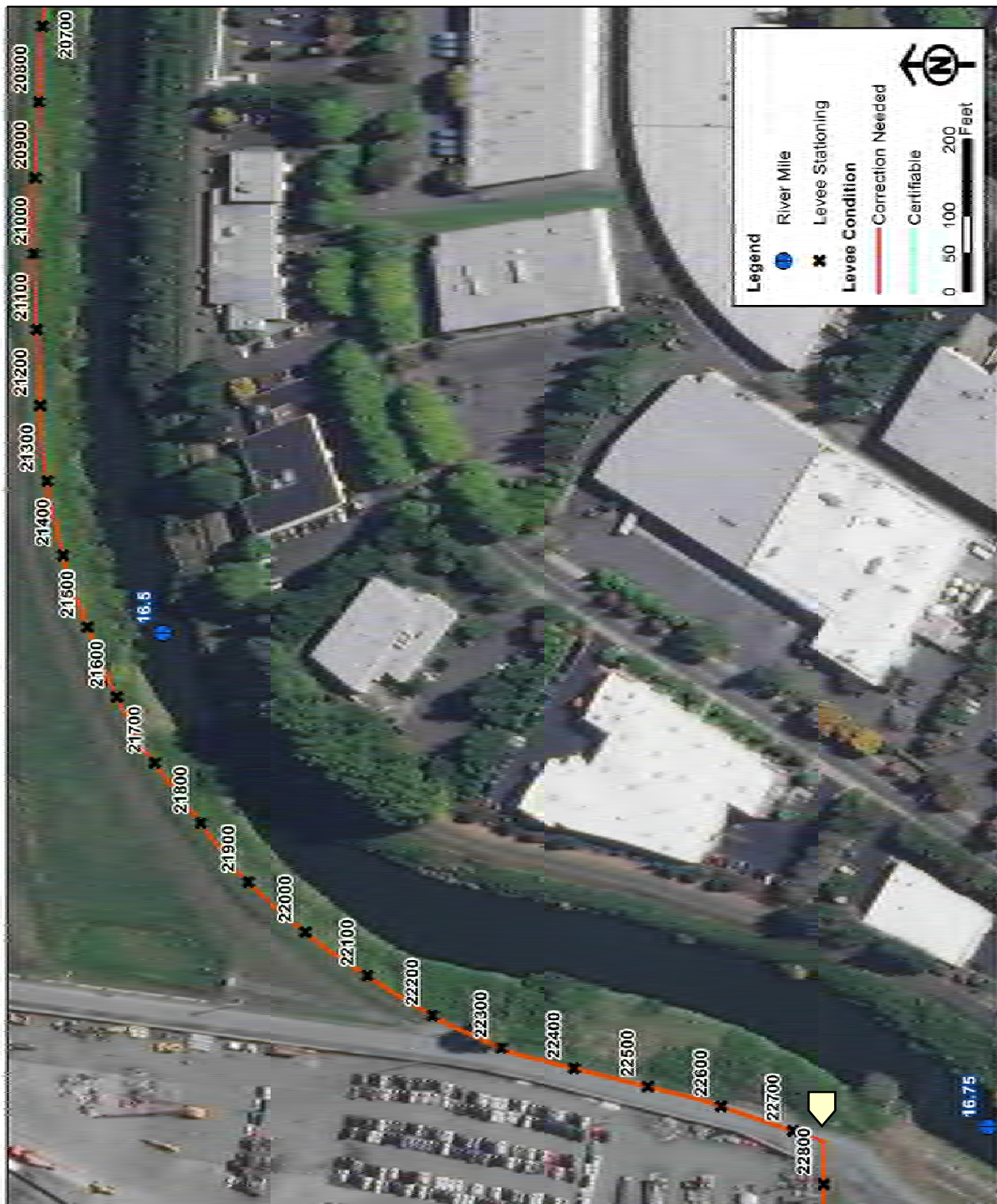
Figure 19. Tukwila Levee segment 18500 through 22750 (upstream portion) that can't be certified in its existing condition.
