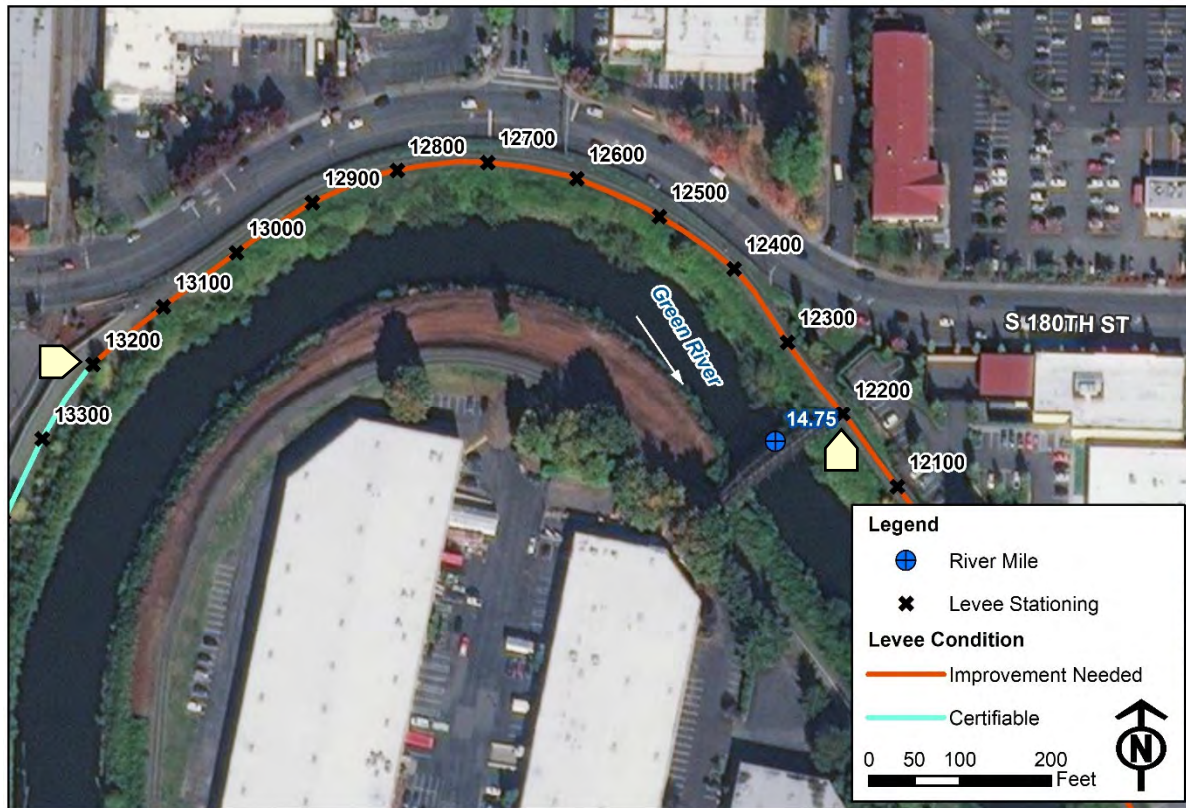
Figure 15. Tukwila Levee segment 12200 through 13200 that can't be certified in its existing condition.
