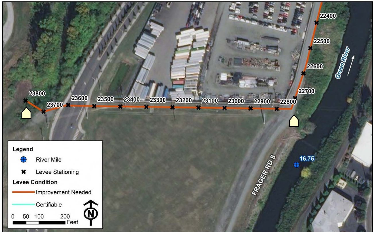
Figure 20. Tukwila Levee segment 22750 through 23800 that can't be certified in its existing condition.
