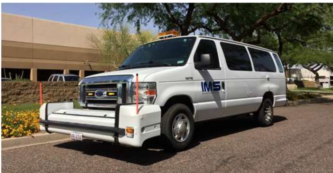
Figure 4 – Laser Road Surface Tester (RST)
