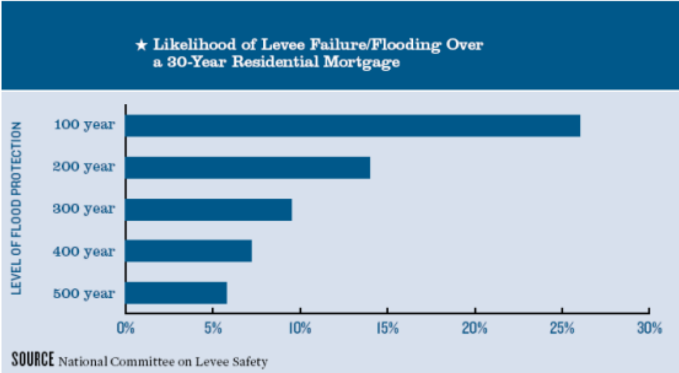
Figure 1. Likelihood of flooding from a 100 to 500 year-flood event during a 30-year period. (From the National Committee on Levee Safety).
