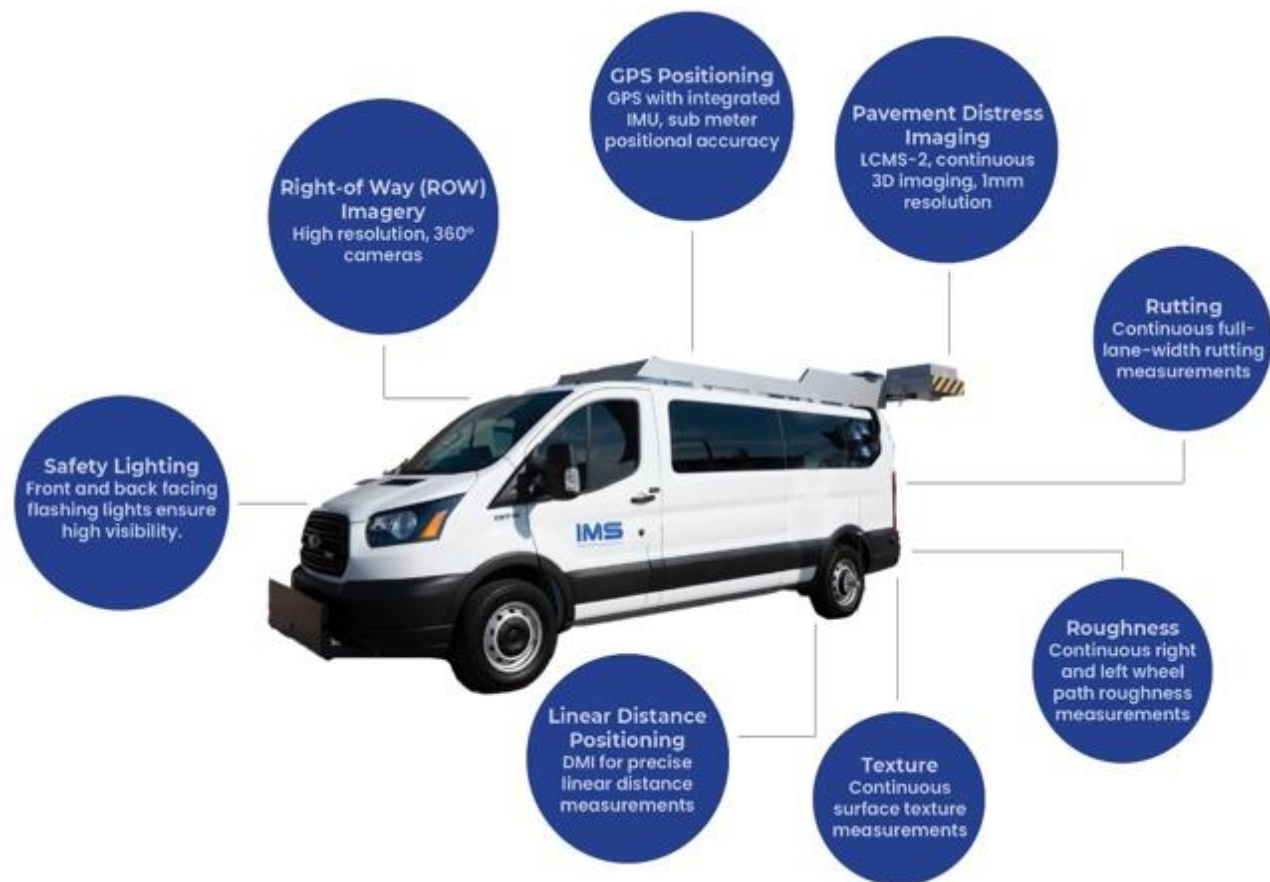
IMS Road Surface Tester (RST) equipped with Laser Crack Measurement System (LCMS-2) (Note: IMS has five RST LCMS-2 equipped systems dedicated to municipal pavement management.)
