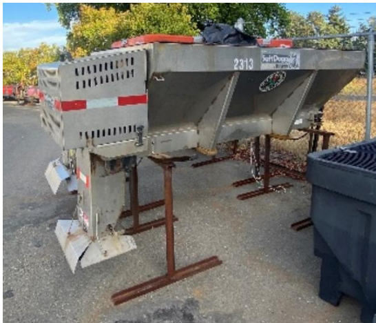
Unit 2313, 2008 SANDER, TRUCK-MOUNTED SALT DOGG 1.8 CU YD 96", MODEL # SCH096SSX. Estimated value: $1,000
