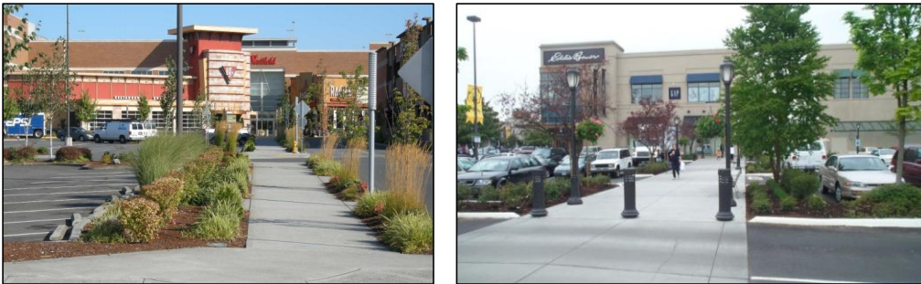
Figure 27 – Site development – pedestrian connections through parking lots connecting street edge to building entrances.
