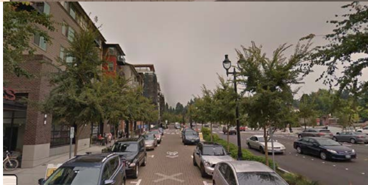
View of the service lane with on-street parking, auto travel lane, and bike sharrows.
